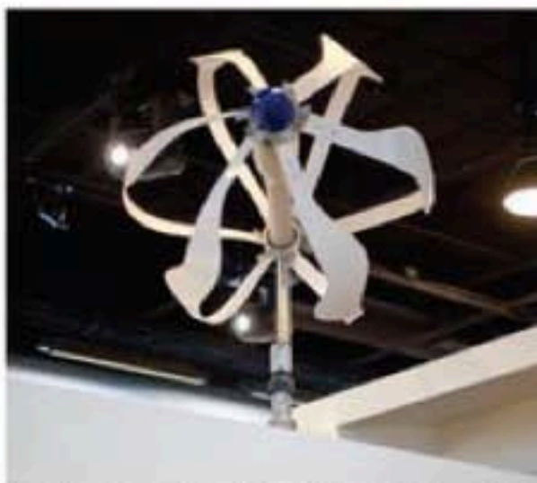
Small garage-top wind turbines designed to catch California's evening seabreeze will mitigate the added power draw from electric vehicles charging in homes at night.
